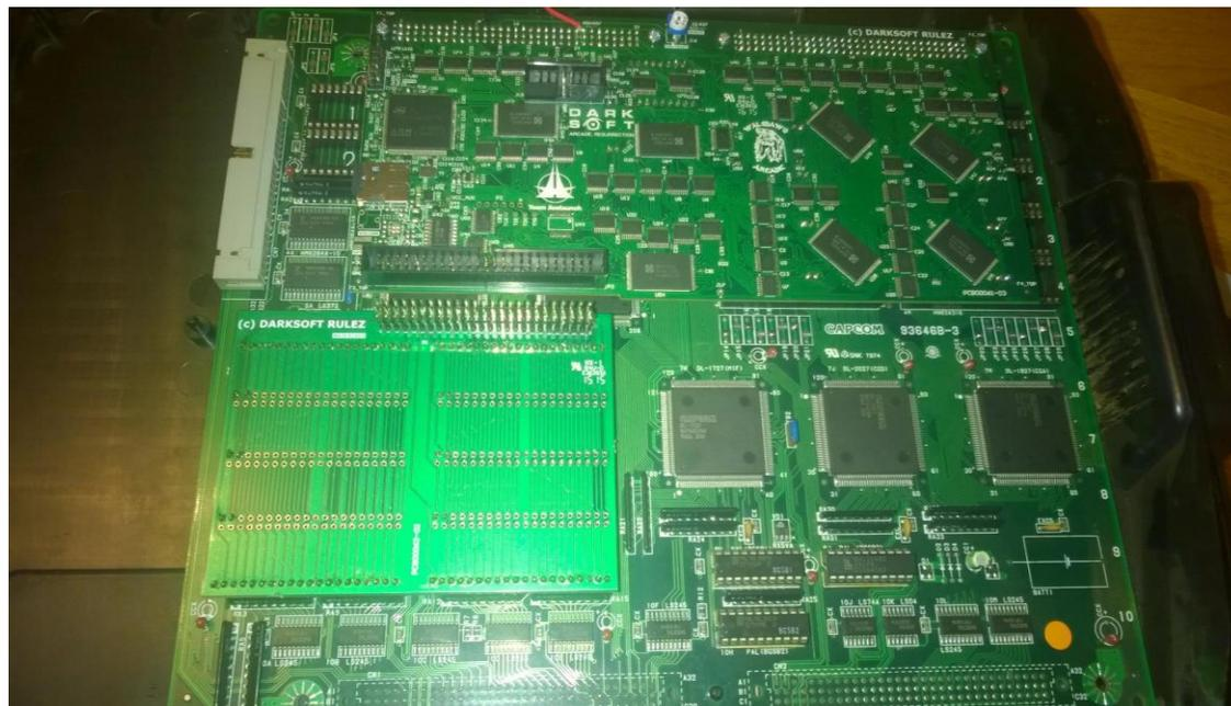
Now you can proceed to insert the tiny PCB that joins these two PCBs together.
