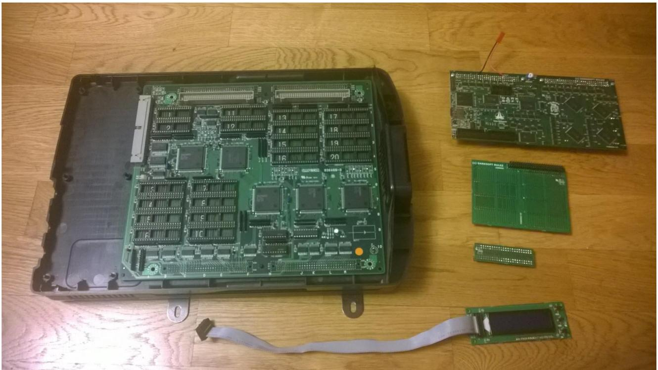
First, proceed to install the smaller PCB. Check that the PCB is placed as in the picture below. First just lay it, to make sure all the pins are in the right place.
