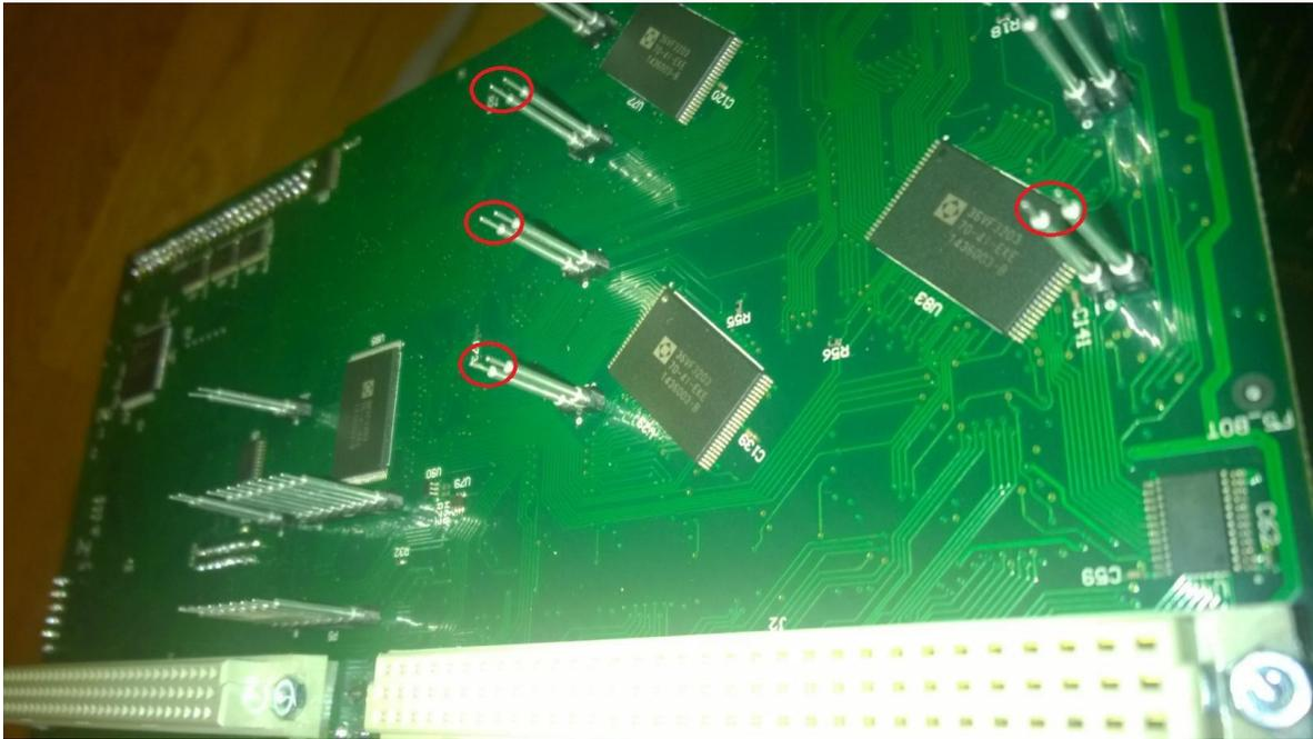
The first thing is to align the white connectors with the ones in the B Board like you can see below. Again you need to carefully look at the pins while you insert them in the Eprom socket to make sure that everything is aligned and the pins insert in the right place.
